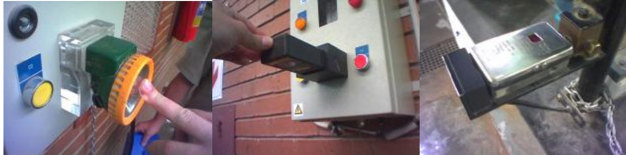
Different types of GDI's being tested and calibrated
